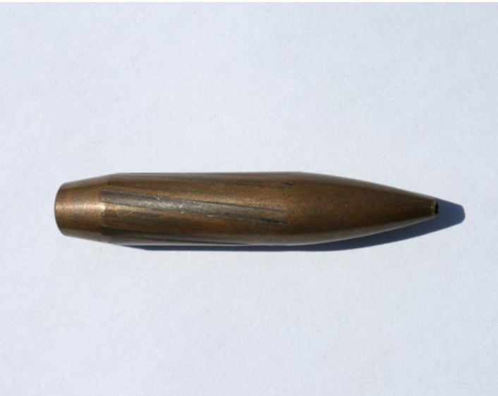
Rifling marks left on a projectile.
