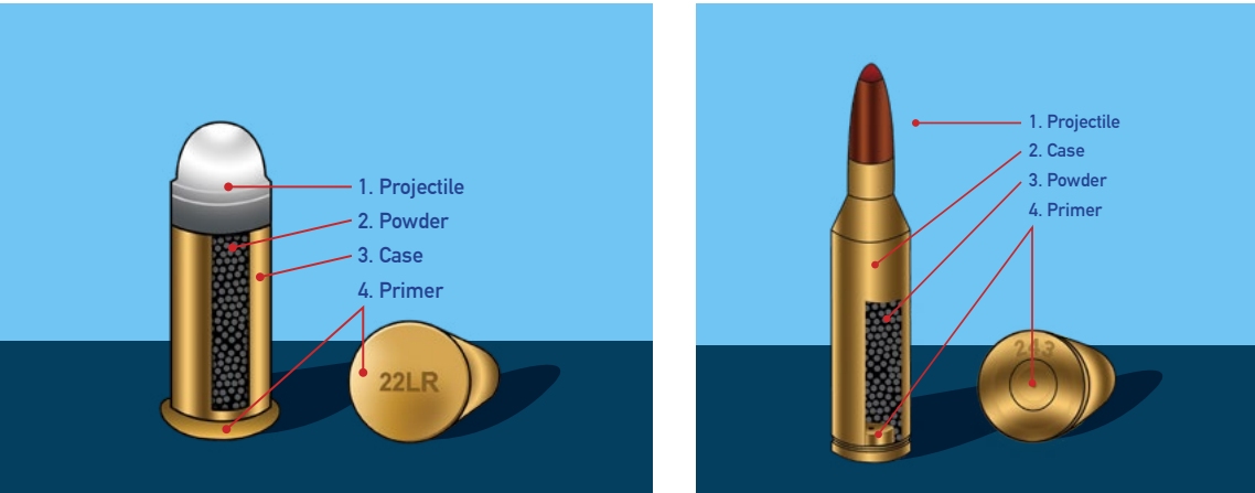
Rimfire and centre-fire ammunition.
