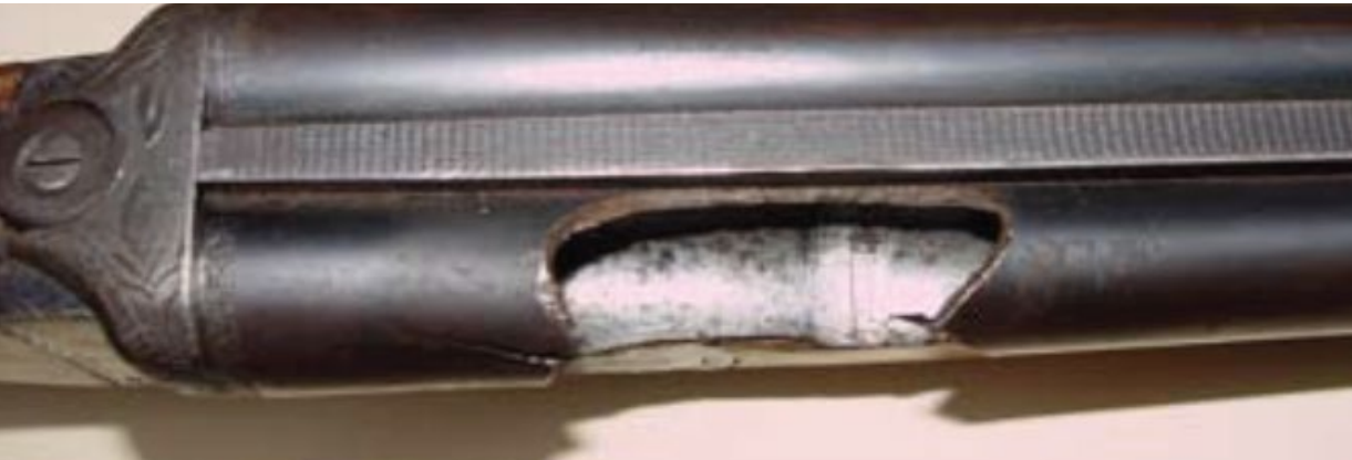
The 12 gauge side-by-side shotgun above was destroyed by firing into a barrel that had been blocked by a wad from a previous faulty cartridge.
