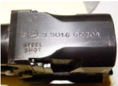
The underside of this over/under (o/u) shotgun breech shows it is suitable for steel shot cartridges.
