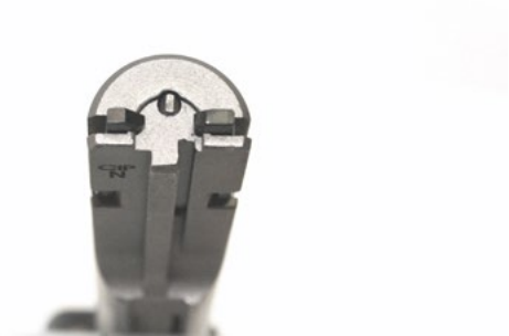
The firing pin of an uncocked rimfire rifle (above). Note the protruding firing pin.
